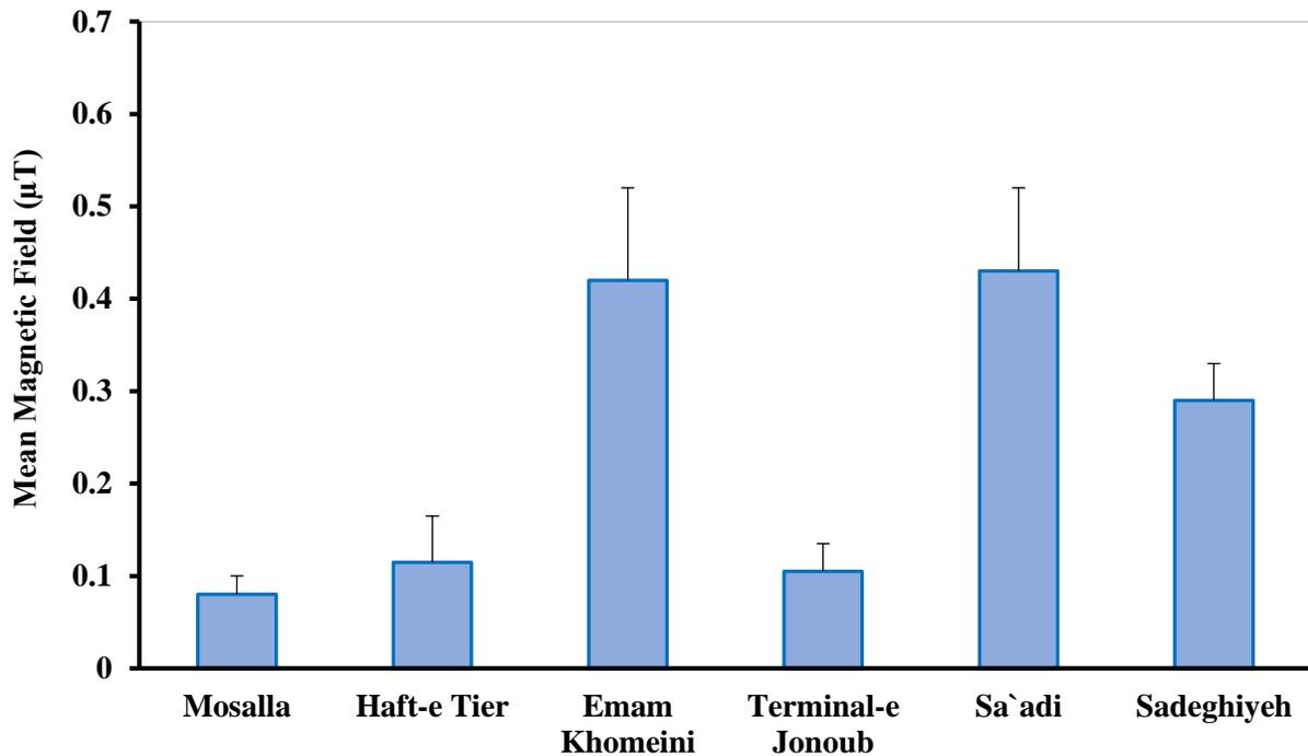
**Figure 2.** The mean electromagnetic field intensity ( $\mu\text{T}$ ) measured at six different metro stations in Tehran on the waiting platform.
