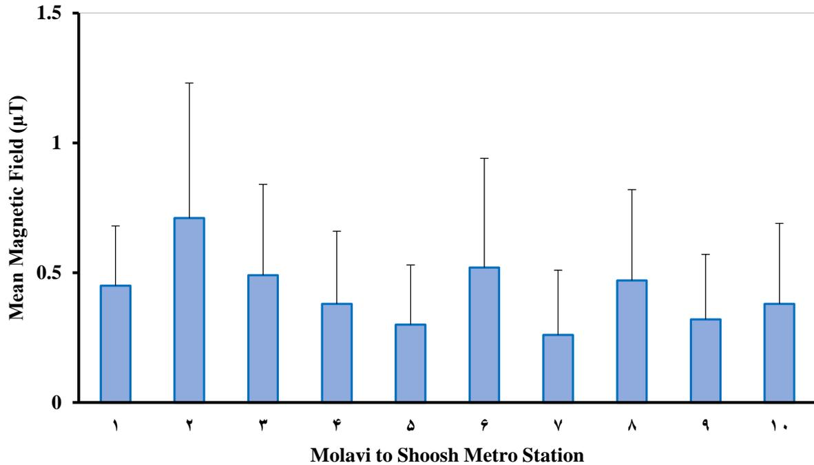
**Figure 3.** The mean electromagnetic field intensity ( $\mu\text{T}$ ) measured inside the moving train between different metro stations of Tehran in the direction of Molavi-Shoosh route.
